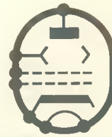
Fig. 4. The circuit symbol for a beam tetrode. The two electrodes between the screen-grid ( g_2 ) and the anode are the beam forming plates. It is common practice to show a connection to one beam forming plate only (as illustrated here) the connection to the other plate being assumed
